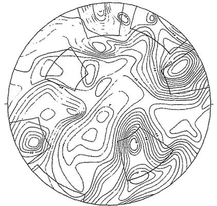
B.-Plot of Horizontal Line Data, Upper Adit; 3249 Fractures, Contour Interval Equals 5 Fractures.
