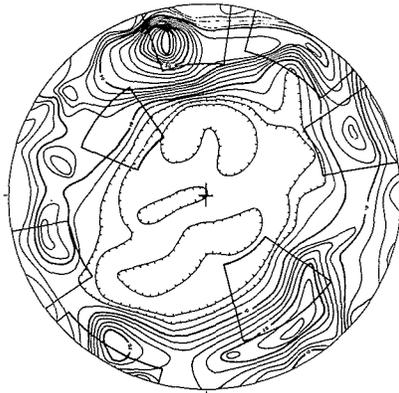
C.-Plot of Borehole Camera Data; 801 Fractures, Contour Interval Equals 2 Fractures.
