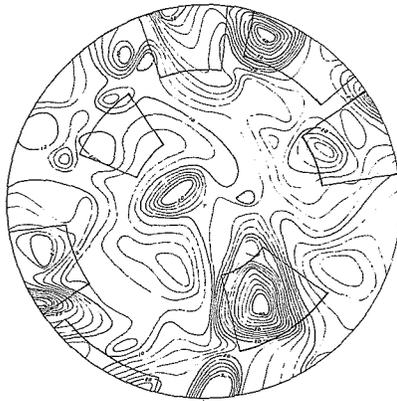
A.-Plot of Vertical Line Data; 1166 Fractures, Contour Interval Equals 2 Fractures.
