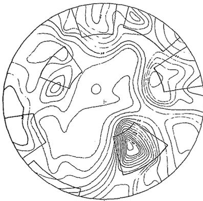
C.-Plots of Horizontal Line Data, Lower Adit; 3916 Fractures, Contour Interval Equals 10 Fractures.
