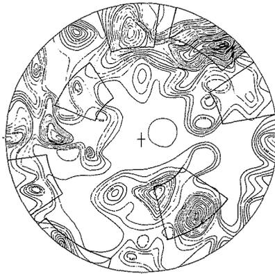
A.-Plot of 211 Fracture Sets, Macro Data; Contour Interval Equals 100 Fractures.
