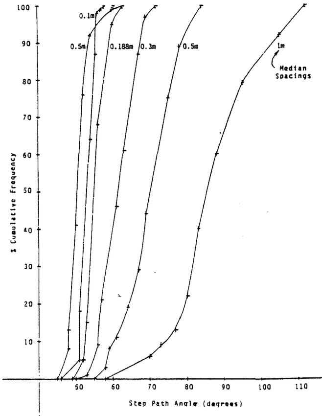
Figure 14. Step Path Angle Cumulative Frequency Curves at Various Median Master Joint Spacings
