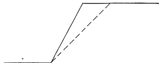
Figure 2. Discontinuous Plane Shear
