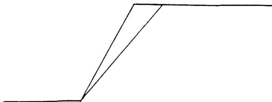
Figure 1. Continuous Plane Shear
