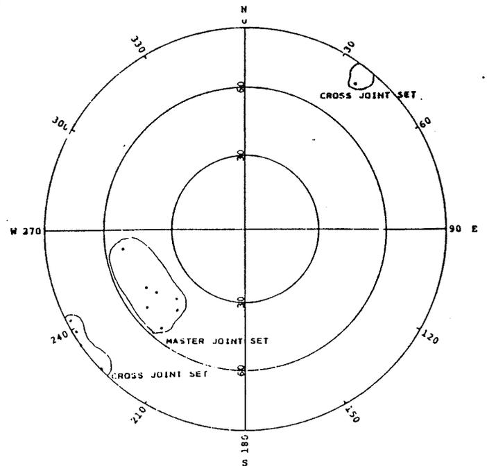
Figure 17. Lower Hemisphere Schmidt Point Plot of Step Path Structure, Bagdad Mine
