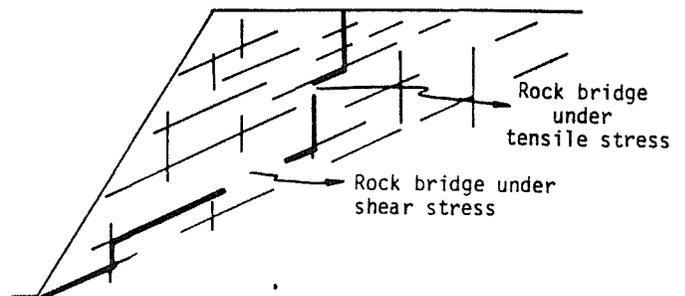
Figure 6. Step Path Separated by Rock Bridges
