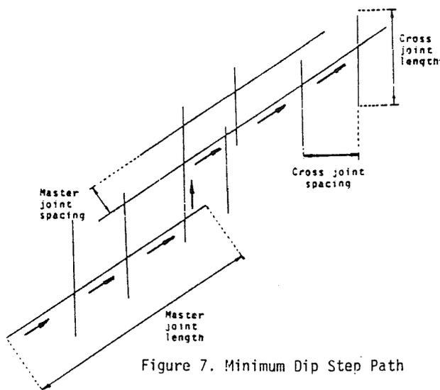
Figure 7. Minimum Dip Step Path
