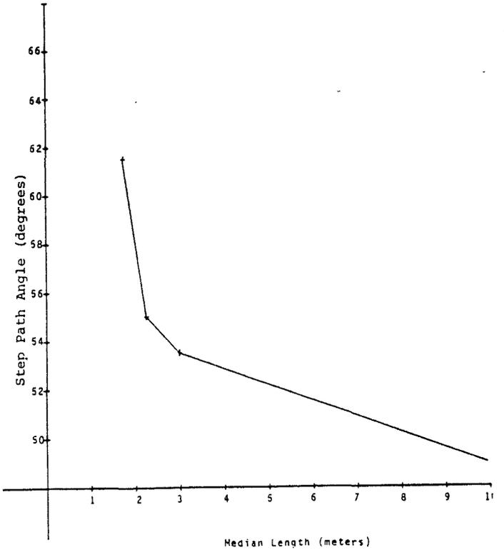
Figure 15. Step Path Angle Versus Median Master Joint Length
