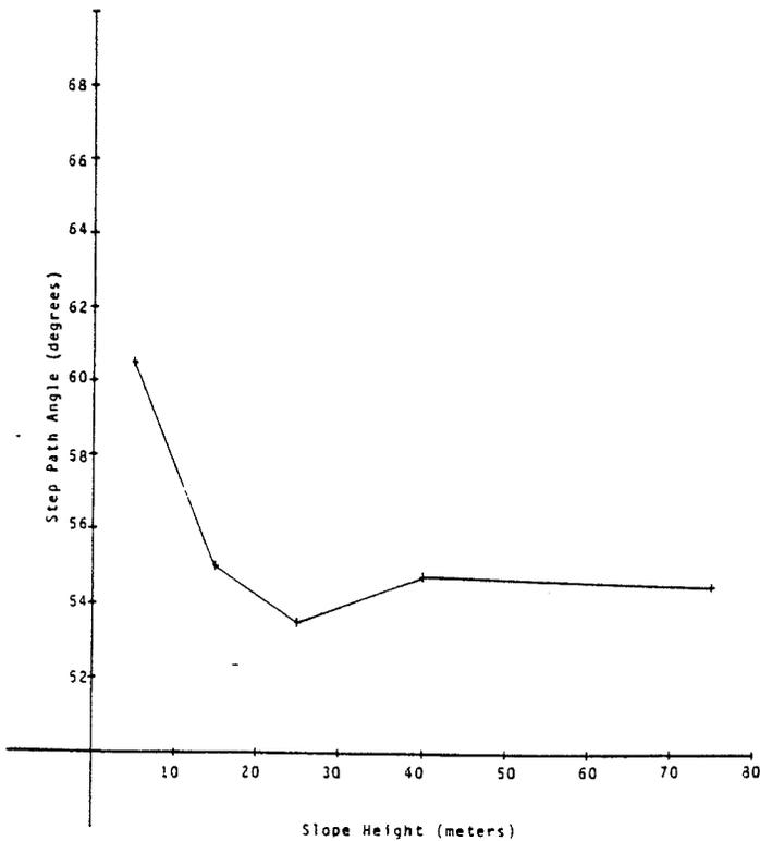
Figure 12. Median Step Path Angle Versus Slope Height
