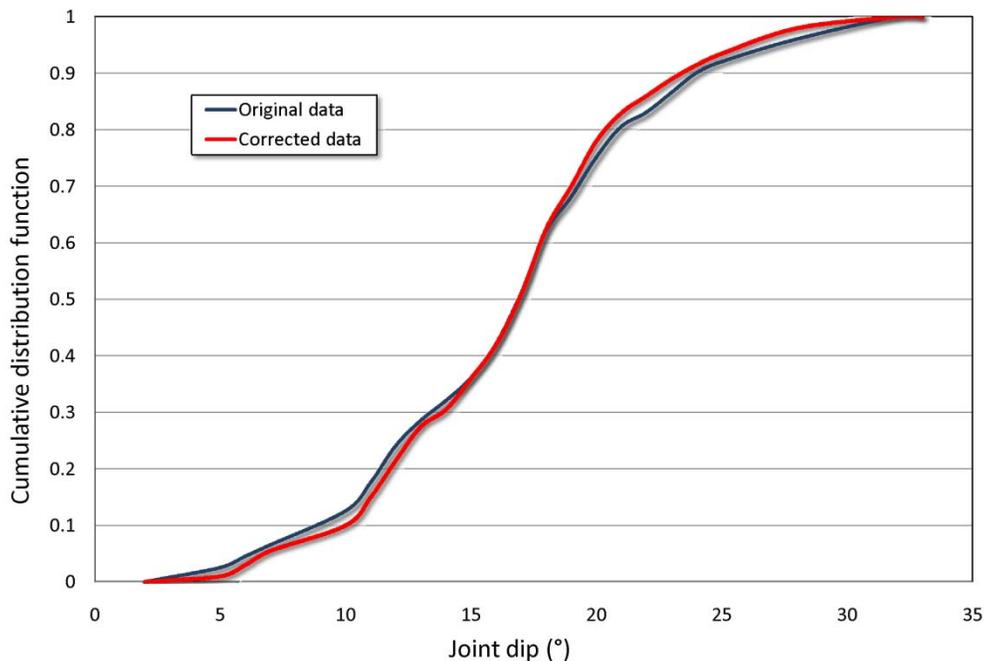
Figure 8. Dip distribution for the bedding joint set before and after the  $\beta$ -angle corrections
