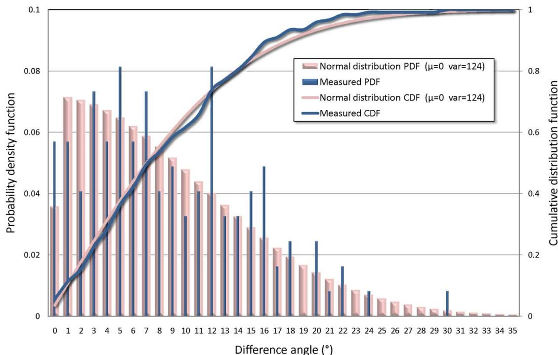
Figure 5. PDF and CDF of measured difference angle distribution and normal distribution fit.
