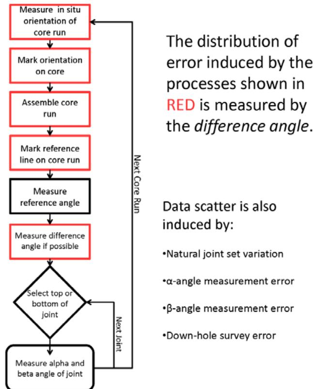
Figure 1. Flow chart of a typical core orientation process.
