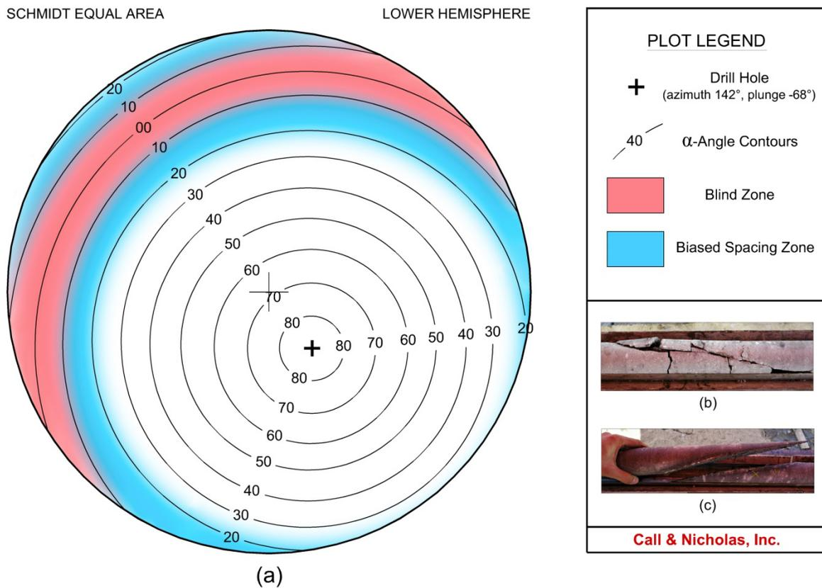
Figure 3. (a) Lower hemisphere Schmidt net projection with drill hole line and corresponding oriented-core  $\alpha$ -angle contours, (b) A damaged joint with  $\alpha = 10^\circ$ , (c) An intact joint with  $\alpha = 10^\circ$ .
