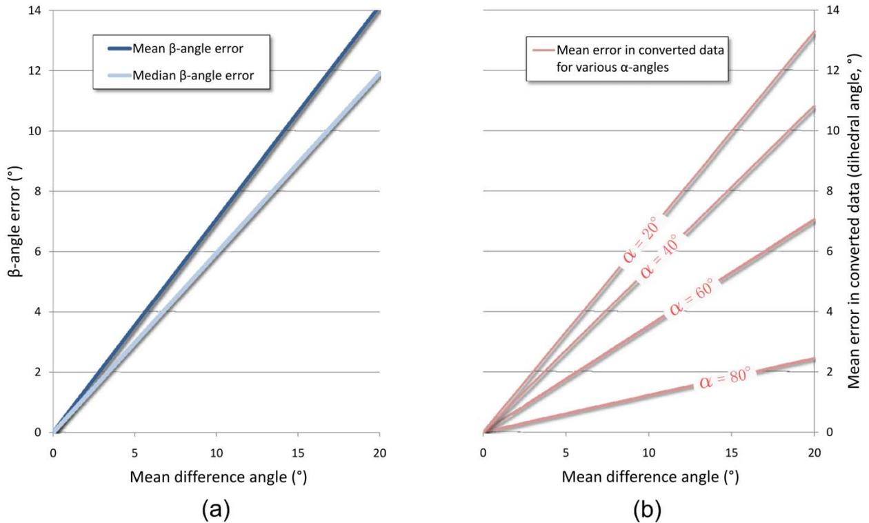
Figure 6. Relationships between the mean difference angle and (a) the mean and median error induced in  $\beta$ -angle measurements, and (b) the mean error in the final converted data measured in dihedral angle
