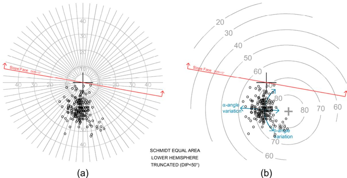
Figure 4. (a) Siltstone bedding joint set poles plotted over truncated equal area Schmidt net, (b) Siltstone bedding joint set poles plotted over the drill hole line and truncated  $\alpha$ -angle contours.
