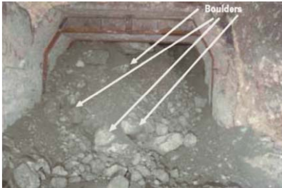
Figure 6. Fines covering large blocks in drawpoint
