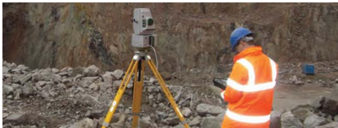
Fig. 5. I-Site 8800 LiDAR Scanner used for wall mapping [8].
