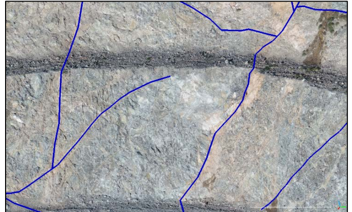
Figure 10. Large scale geologic mapping of faults exposed in bench faces using a true-color point cloud.
